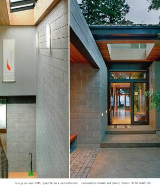
A large east-west CMU 'spine' forms a central thermal score for the house. This massive wall cuts down temperature swings and is aligned with the operable skylights to take advantage of the cooling techniques. The wall doubles up to divide the private and public spaces. The north, the private portion of the house, is much more
